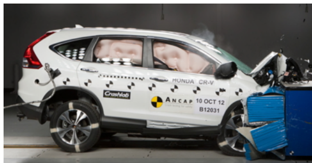
Offset crash test at 64km/h
