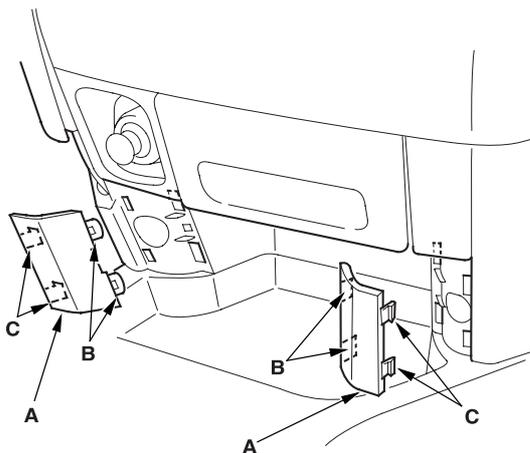
4. Remove the screws (A) and clips (B) from the dashboard center lower cover (C).
