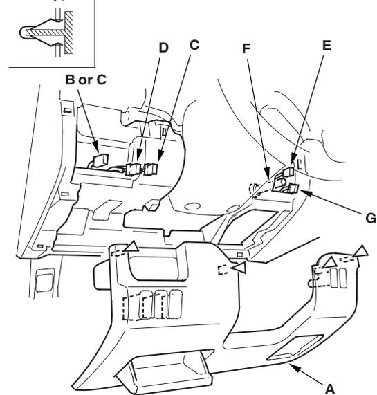
**4. Install the cover in the reverse order of removal, and make sure that each connector is plugged in properly, and the air hose is connected properly.**
