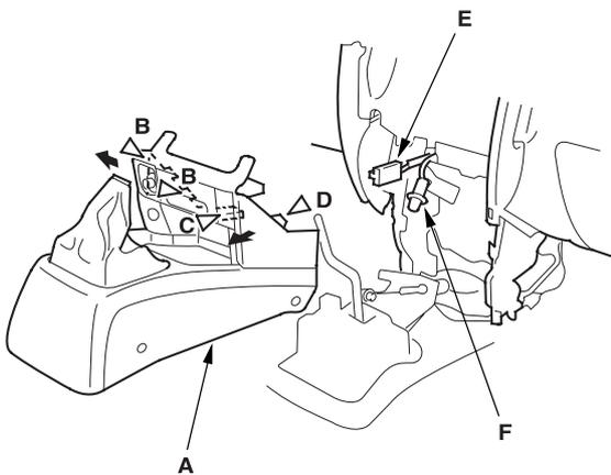
6. If necessary, remove the screws, then separate the center console (A) and center lower cover (B).
