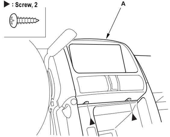
2. Pull out on the bottom of the dashboard center panel (A) to make create a gap between the dashboard and panel. Gently pull out along the panel to release the clips, then remove the panel. Disconnect the hazard warning switch connector (B).
