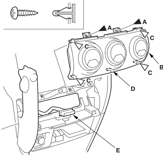
4. Install the panel in the reverse order of removal, and make sure the heater control unit connector is plugged in properly.
