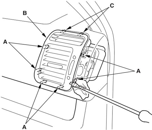
2. Remove the vent by releasing the hooks (C).
