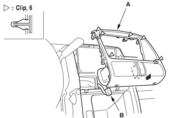
3. Install the panel in the reverse order of removal, and make sure the hazard warning switch connector is plugged in properly.
