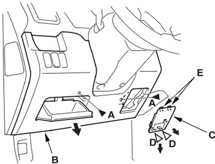
**2. Pull out the bottom of the driver's dashboard lower cover (A) to release the clips.**
