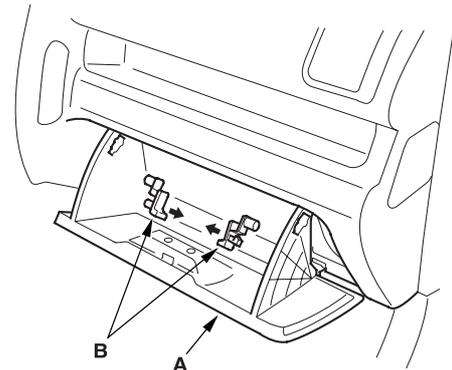
2. Remove the bolts, then remove the glove box (A).
