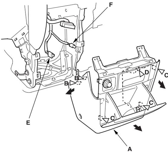
4. If necessary, remove the pocket (A) from the dashboard center lower cover (B).
