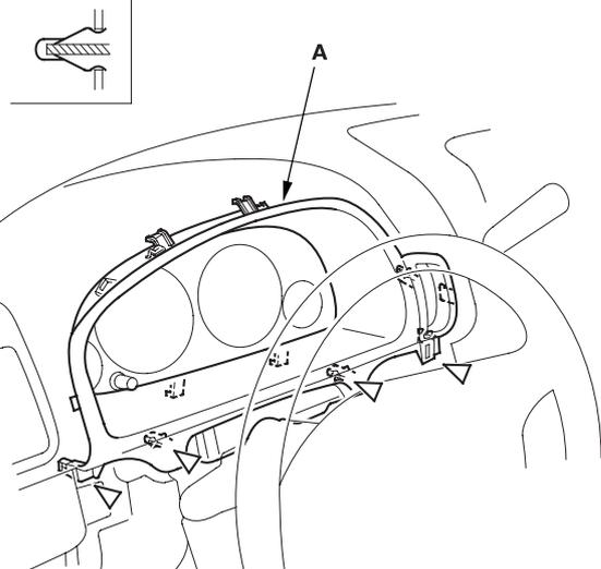
4. Remove the instrument panel (A).
