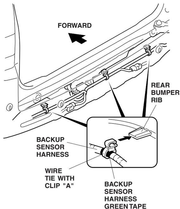
37. Using one wire tie, secure each center sensor 2-pin connector to the backup sensor harness.
