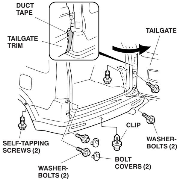
7. Remove the center clip, and remove the self-tapping screw from each side of the rear bumper.
