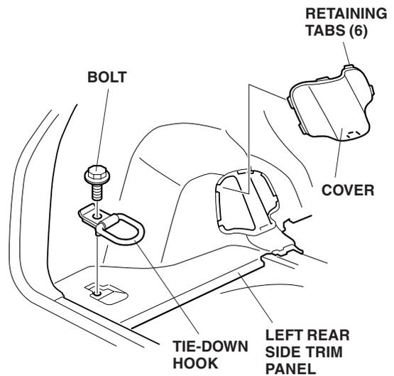
16. Remove the cover from the left rear side trim panel (six retaining tabs).
