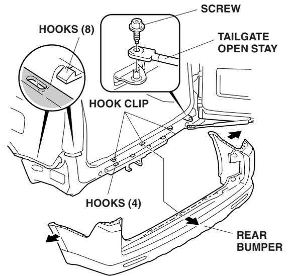
9. Open both sides of the rear bumper, disengage the hooks and remove the rear bumper by pulling it outward. Be careful not to hit the bumper against the tailgate. Set the rear bumper on a blanket.
