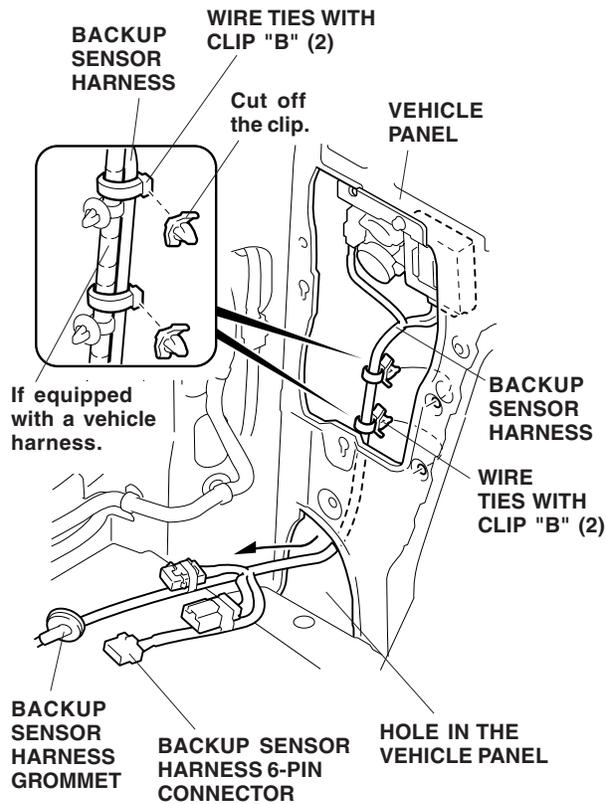
29. Using two wire ties with clip "B", secure the backup sensor harness to the vehicle panel. If there is already a vehicle harness using the two vehicle panel holes, cut off the clips from the two wire ties, and secure the backup sensor harness to the existing vehicle harness.
