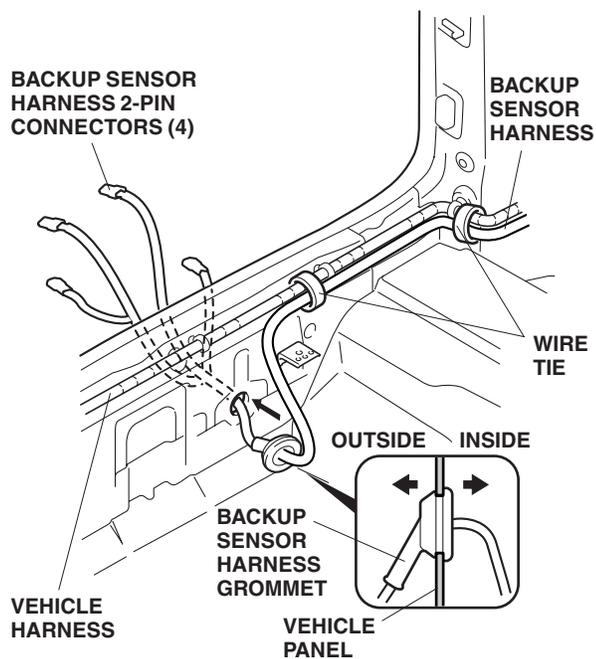
34. Using two wire ties, secure the backup sensor harness to the vehicle harness.
