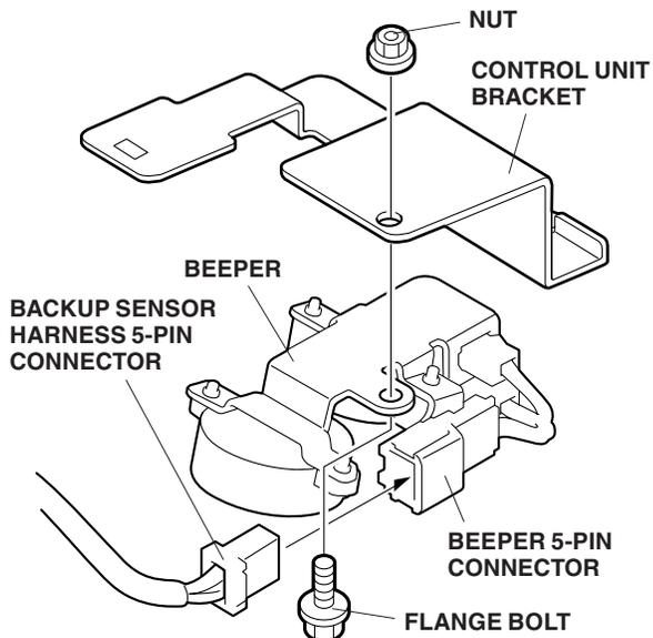
24. Plug the backup sensor harness 5-pin connector into the beeper 5-pin connector.
