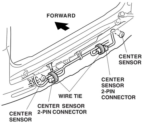
38. Attach the clip to the backup sensor harness at the location, then secure the harness to the boss on the rear bumper using the self-tapping screw.
