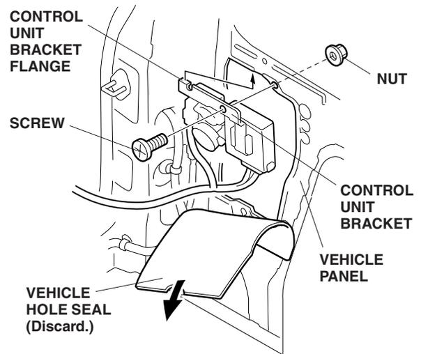
27. Position the control unit bracket on the vehicle panel, and install the screw and nut while pushing the control unit bracket flange against the vehicle panel. Tighten the screw and nut securely.
