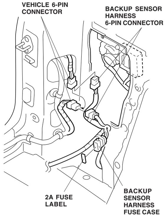
31. Unplug the taillight 6-pin connectors, and plug the backup sensor harness 6-pin connectors in between the vehicle 6-pin connectors you just unplugged.
