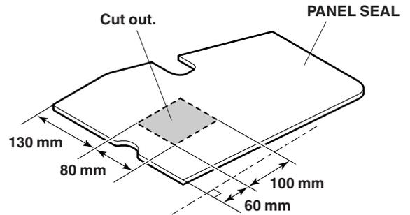
41. Align the panel seal over the beeper on the vehicle panel, and attach the panel seal by removing the adhesive backing.
