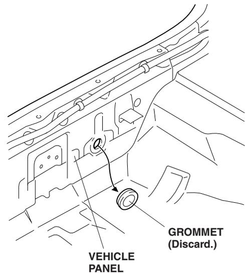
33. Route the four backup sensor harness 2-pin connectors through the vehicle grommet hole from the inside to the outside of the vehicle. Install the backup sensor harness grommet in the vehicle panel securely.
