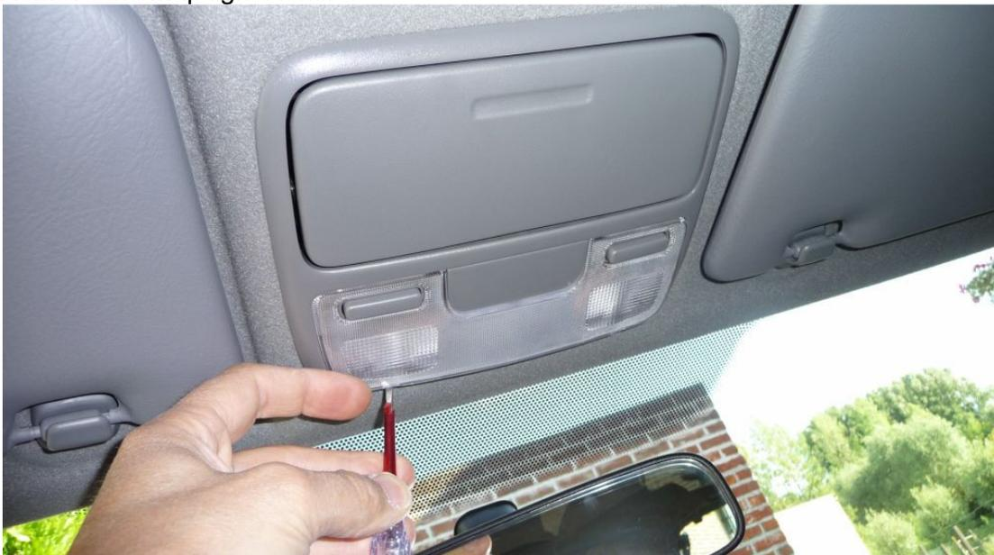
Remove the map light fixture, release 4 screws, remove the fixture, then disconnect the 2 wire connector
