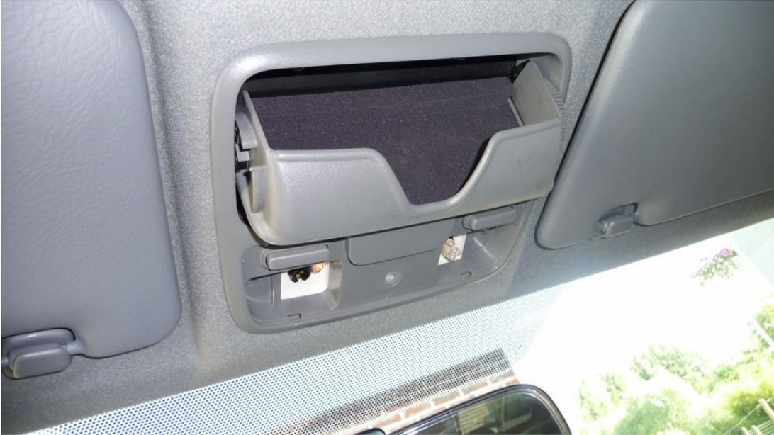
Remove the centre light and pull the wire, release a bit the sunroof sealing.
